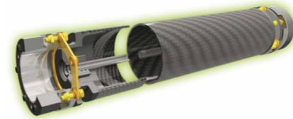
ROBA®-DS with 2.5 m long sleeve (CFRP), with integrated cooling lubricant feedthrough, suitable for speeds up to 10,000 rpm.
